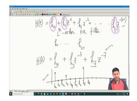
So, instead of h l if it is a filter. So, obviously, I can have some sort of a transfer function of it right. If it is a system of linear equation I can get a transfer function of it. So, this H Z is the Z transformation of that individual h l. So, what does it mean? I can say this is nothing, but h 0 will be there plus h 1 Z inverse plus h 2 Z inverse 2 plus dot dot dot. Say I have considered up to l number of taps because beyond that I do not see any more taps coming up ok.
