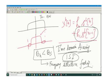
So, if I have a bandwidth of a signal bandwidth of a signal this is my say transmission bandwidth and after I do a reception it is gets shortened the bandwidth is shorter. What is the time domain impact? Time domain impact is that you will naturally see some sort of an aliasing because some of the components are lost right some of the components are lost.
