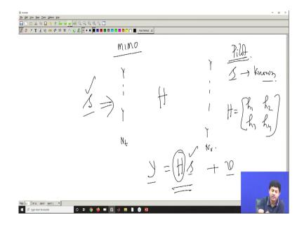
So, for example, I have a basic MIMO ok. So, because if I explain it for MIMO. I just give a touch upon so that it can be extended to the larger hybrid beam forming case as well. See, if it is a MIMO case, you have this N t antenna here N r antenna here right. So, what is the data model; if this is a channel H into s plus v that is a standard data model right see if I feed s here ok.
