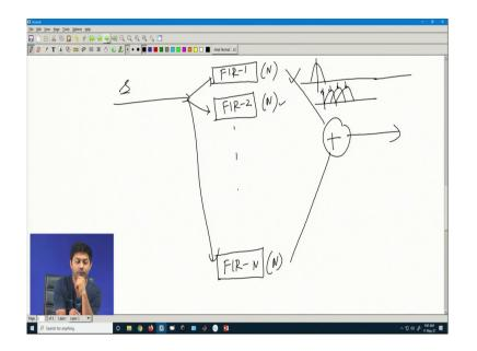
So, which means that your OFDM is nothing but so you have a data which is your s vector. So, there is a first filter, there is a second filter and there are nth filter nth FIR filter and each and every filter has a length N. This also has a length N, this also has a length N. So, the data goes everywhere and that is precisely I mean multiplication also shows the same thing.
