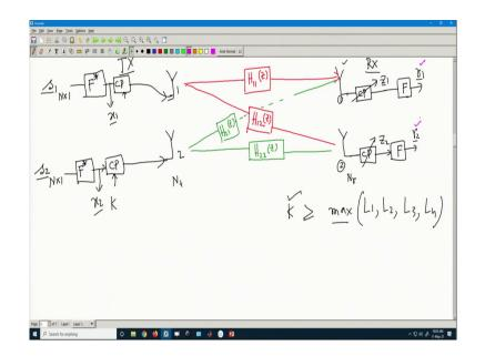
So, this is my antenna number 1; this is my antenna number 2. So, the first thing I do here at individual is I discard the CP here. Also, I discard the CP. What I received Z 1 vector, here I receive Z 2 vector, then what I will do is, I do the FFT. FFT I do, FFT operation here. Also, I do FFT operation. So, I multiplied with the F matrix I should naturally guess R 1 vector here R 2 vector.
