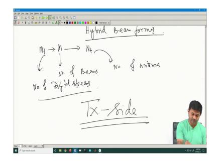
So, now, let me draw let me use this term hybrid beam forming directly hybrid beam forming. So, what we have learnt it here? So, we have learnt it M t digital symbols or M t digital stream data stream goes through a digital precoder, where it converts to M number of data stream and then it gets converted to N t number of you know antenna beams.
