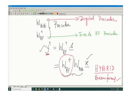
So, this whole thing this W BB and the W RF t both of them are called precoder. Why it is called a precoder? Precorder is its kind of some matrix manipulation of your data at the transmitter side. So, that is as simple as that that is your precoder right. I mean it is doing that job right fairly if you can understand.
