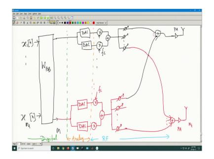
So, let us take I have x here ok and I have x M t n here ok. Now this data this data goes through matrix multiplication that is easy in a digital system I have n number of data and that creates M number of data here its pure digital ok. Then what happens? Then it goes to DAC.
