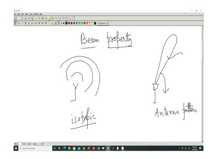
So, these are the beam property. So, when you say beam so it is mainly the electromagnetic wave propagation. So, definitely it is in the air not inside the antenna. So, this is an antenna so when I say beam it is basically this I am talking so these are my radiations.
