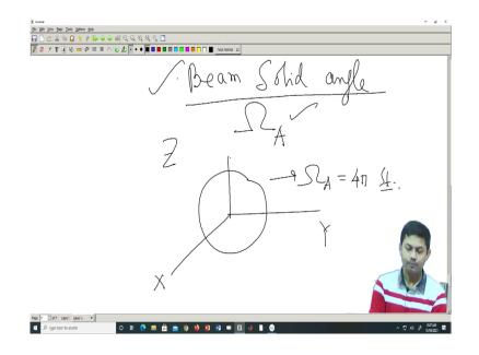
Now, there is one more aspect comes that is called beam solid angle it is a another parameter that we should know ok. So, what is beam solid angle? Beam solid angle represents, how much solid angle is occupying the actual power is something like that ok. And it is a very important parameter for a beams it is called beam solid angle. Say for example, I have a X Y Z, X Y and Z; let us say my antenna radiation is like a ball ok.
