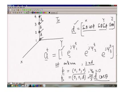
If you look at what is there in X? This is the X coordinate part, this is the Y coordinate part, this is the Z coordinate part; this is my X coordinate part, Y coordinate part, Z coordinate part of my direction of departure or the angle of departure. So, that mean as if like I am standing at
