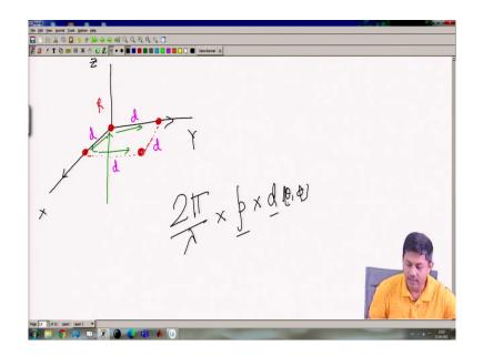
So, this will be applied so many places, this concept, 2 pi by lambda just understand the phase difference among these antennas are nothing but 2 pi by lambda into antenna position vector multiplied by the direction of either arrival or direction of departure or it is a position where you stand it, the general position ok which is a function of theta and phi. So, this is the crucial part ok. So, I am just trying to show you various applications on that. So, let me remove this part ok.
