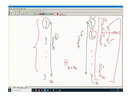
So that means my third configuration will be when I have multiple antennas in the T x side will have multiple antenna in the R x side ok. So, let us try to understand that, from this side I will get h vector corresponding to t from this side I will get h vector corresponding to r. That mean h bar t I will get it as if like I have only 1 receiver, h bar r I will get it as if like I have only 1 transmitter, now let us combine it ok.
