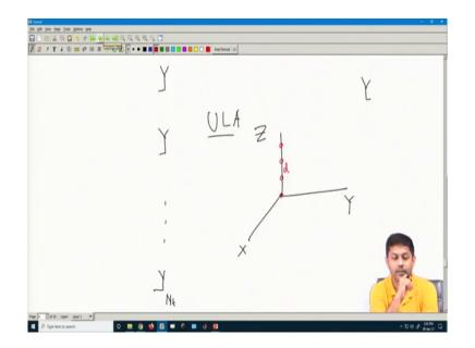
This is the first antenna this is the second antenna and I have N t number of antenna here, but at the receiver I am having only just one antenna it will be easier. So, in the first case one transmitting antenna multiple receiving antenna, in the second case we are starting with multiple transmitting antenna but one receiving antenna, then we will combine it together it will be easy for us to do.
