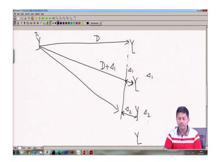
So, what I mean to say here so, this is my receive antenna, this is my receive antenna and this is say some other receive antenna, I am at the rx side. So, the distance I am only assuming here currently that it is sent from one antenna so, this is going here, see if this length is D, this length will be D plus as we said some notation I have used here, some delta i we have used that notation.
