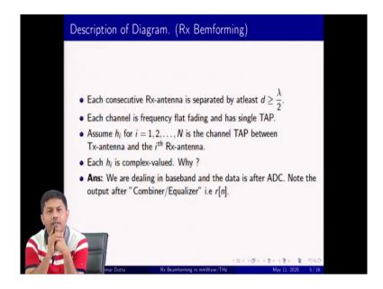
Let us see what happens. And this is some more assumptions. And each Rx antenna is that the distance is d, assumed to be d. So, that means, the distance here that this antenna the first antenna to the second antenna the distance is assumed to be small d not the capital D. Capital D is the distance from the transmitter to the receiver antenna structure.
