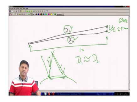
So, from here from this antenna, so there is an antenna here there is an antenna here, and the distance is D 1. From this antenna, there is one more antenna here ok. This distance is D 2. And I am assuming a far field and this distance at least lambda by 2. Now, think of a scenario say I am operating at 60 gigahertz. So, what is this lambda? Lambda is 5 millimeter; lambda by 2 is 2.5 millimeter. Imagine 2.5 millimeter the distance between this antenna and this antenna.
