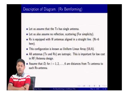
So, basic few assumptions that we have assumed here. I just reiterate what we have learnt it that Tx has single antenna, and no reflectors and scatterer for simplicity. Then we will bring it back, finally, that is what our millimeter wave part. And Rx has you have in this case 6 such antennas.
