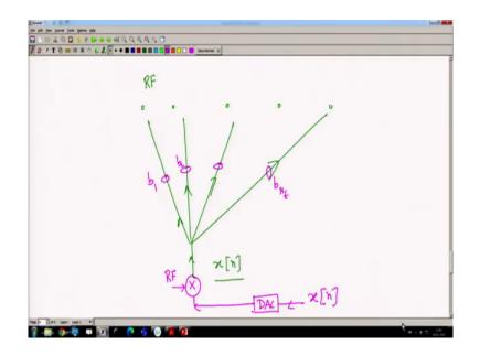
So, this is where we left it in the last class right. We saw that this is the actual architecture from the transmitter side where we have the x n, then you have a DAC, then it will have an RF. And from that from the RF, it just spread across multiple antennas for the beam forming purpose right. And then we saw that in between there will be some multiplying coefficients, and then we have to understand why they are exactly.
