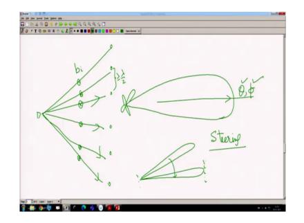
Now, let us say I have these antenna configurations and there may be one more. Let us assume that. So, if I feed them directly physically I am just connecting the RF data directly here. So, what is the consequence? Consequences that will form a beam, it may form a beam depending on how exactly the antennas are placed, and what is the phase difference and so on. We will explain that.
