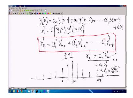
So, it would be, so let us write down the equation first y n, you have a 1 y n minus 1 plus a 2 y n minus 2 plus dot dot dot. What will happen? a p n minus p, this is the definition, plus e n. This is the typical definition, right. Then what is our job? Our job is to calculate the gamma k which is equal to E of y n. So, this is typically I will be doing it; n plus k. That is my job is, right.
