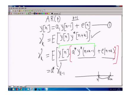
So, let us say I am taking the autoregressive model. So, autoregressive p model, ok, AR p model. And we will try to find out how you can estimate or how you can determine the exact coefficient and how you exactly estimate the complete autocorrelation function. So, let us say my sequence is y n, let us say its standard y n sequence.
