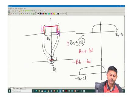
So, which means that as if like you have a spectrum this red spectrum ok, it just keeps sliding left and right; left and right depending on how exactly the Doppler is there. So, there will be left shift or there may be there may be right shift or there may be a left shift ok. How much it will shift? That depends on the on the velocity of the system.
