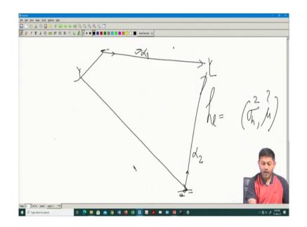
The logic is that you have a transmitter here you have a receiver here you may have a reflector here you may have a reflector somewhere here bottom of my screen. So, the guy which is closer to it will always pump you larger power compared to the one which is here right. So, this will be a kind of a weak fellow this will be kind of a bigger fellow.
