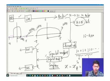
Then this signal which has come from the digital filter, which is a higher order digital filter, but with a very you know sharp transition, but it has a higher rate of signal. So, what is the consequence of it? So, it means that my spectrum will now be like this; this is pi to minus pi, but now the spectrum will not have any extra component because I have used a very sharp digital filter.
