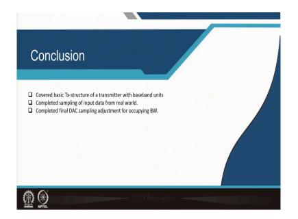
So, we have covered so, far the basic structure the of the Tx and then how to do the input bit input data sampling from the real world like how to get it through the ADC and then adjust the sampling rate and then finally, when it goes to the Tx just before the RF part how it changes the sampling rate again back to the DAC for readjustment of the bandwidth occupation.
