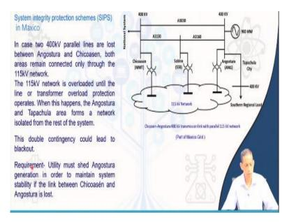
Let us see an example how in Maxico grid SIPS using synchrophasor data is being implemented. So, this is a part of Maxico , Angostura and Chicoasen, this 400 kV line they are parallel lines, double circuit lines and there are number of connections for the 100 kV line and that 115 kV network. So, what happens that this 900 MW generations possess power to the national grid and other portion of the system through double circuit line and also there is a connection of 115 kV line also.
