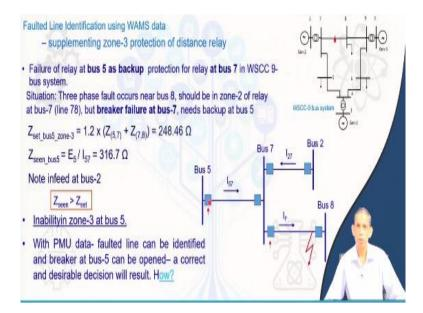
Now next we will go for another applications in real time perspective how the corresponding PMU data can supplement the zone 3 protection for better decision. In this perspective we say faulted line identification. So, what do you see that any line having a fault in this 9 bus system can be identified from different measurements of the PMUs, then we can use that for the backup protection also.
