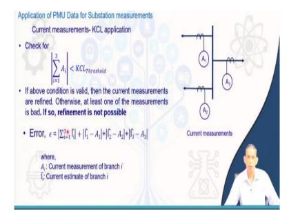
Similarly, in a substation we can have this corresponding current measurements and in current measurements we can apply Kirchhoff's current law, then this current law can be used for checking whether measurements are correct or not. So, some of the current measurement at a bus with all measurements coming to this bus. Ideally, this summation is close to 0 and is less than a threshold, then we declare that the measurements are okay, otherwise we suspect.
