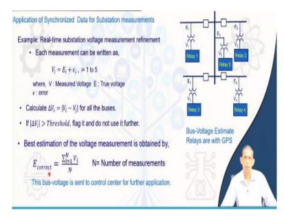
Now furthermore in second application we will see how synchronized data in real time can be used for substation measurements for the accurate information at the substation levels. Two aspects, one is the voltage another is the current. So, first we will see that how voltage measurements can be obtained in a better way at a substation.
