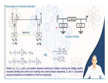
Let us come to different applications we will go one by one. First one is transmission line parameter estimation using synchrophasor data (synchronized data), data from the PMU. Note that these we have already address that these synchronized data or the phasor measurement unit data which can be availed from the relays with GPS facility.
