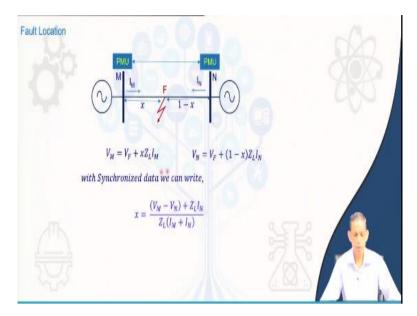
Fault location we have seen in travelling wave perspective so there also we mentioned about if we have synchronized data at both the ends from PMUs application, fault location is offline business there is no issue of speed. So, in this case, if we have a fault at *x* so then we can write down this side single phase synchronized basic equation if you write and then we can extend to three phase concept also. The voltage and current relation at bus M can be written as
