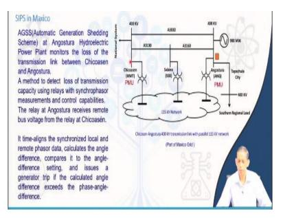
So, what is being done we see here that we have a PMU place at this end and we have PMU at this end through available region with GPS facility. Now this PMU sends data information to this one in real time to communication system and the corresponding voltage data here and voltage data are here they align and then from the alignment the processing processor here does sees that what is the angle deviation between this side and this side.
