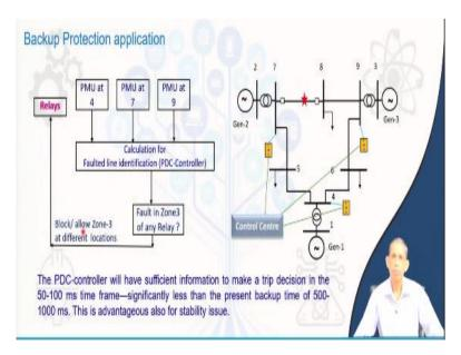
Now what do you see that this is the 9 bus systems and we have PMUs we collect at a control center to this PMU and this control center can process the corresponding PMU data, align them
