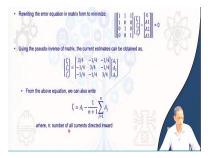
So, with that error if we write that corresponding error equation in matrix form,
