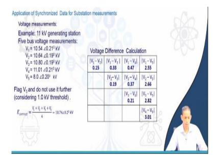
We will see an example on voltage measurement at 11 kV generating stations we have 5 bus measurements like that what we see. So, these 5 meters, relays, PMUs they provide  $V_1$ ,  $V_2$ ,  $V_3$ ,  $V_4$ ,  $V_5$  at one instant of time one loading conditions are given by
