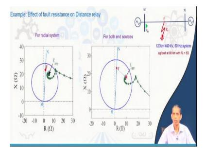
Now, let us take an example now. We have a 2 bus system 400 kV line 120 kilometer and we created a fault 80 kilometer from the RM phase-a-to-ground fault with  $R_f$  equals to 5 ohm only. In real situations it may be much more also. So, what we say that for a radial system we see the corresponding fault deviating from the line you can say that impedance line this much settling here with that 5 ohm.
