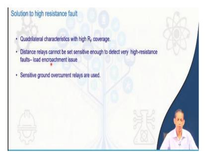
So now if the fault resistance becomes a prominent thing particularly for the phase-to-ground fault then the modulus apparent impedance then what is the solution for that? So, one is that the quadrilateral characteristics can be extended with high value of  $R_f$  so that the area coverage becomes more, but if we consider for this larger zone having, we can say that characteristics larger radial like zone 3 or so.
