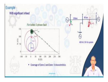
As an example this is a case to 250 kilometre first line, in the second line at 80 kilometre 3 phase fault is created and what you see that this is 80 kilometre in zone 2 of this relay, but if you see the corresponding fault to be beyond zone 2 it settles in zone 3. So, this clearly says that we can say that the apparent impedance seen by the relay is higher than expected we can say that it should be F point.
