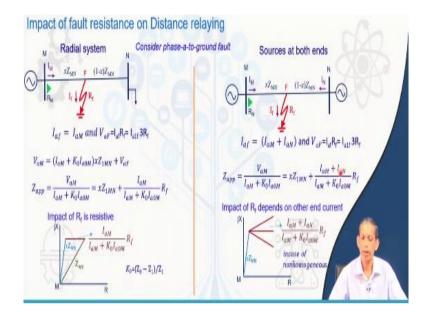
So, going further on this we will see how the effect of the fault resistance in different situations affect the distance relay. We see that this fault resistance is of significant value or phase-to-ground fault compared to phase-to-phase fault. So we will analyze the phase-to-ground fault. Let us consider phase a-to-ground fault for this simple 2 bus system. So this is a radial system power is flowing from bus M to N.
