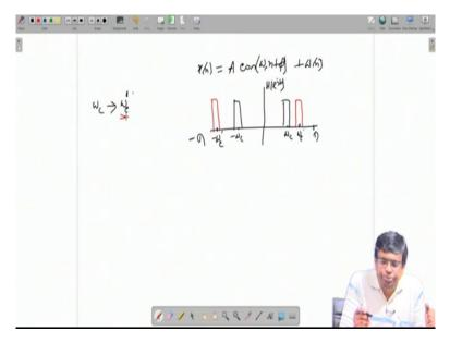
Okay that is digital domain when we have got a single x n which has got some a Cosine some constant, you know, digital frequency plus some phase phi and some noise w n. W n is noise, white noise with I mean appreciable noise power. So this signal is buried in noise. You want to recover the signal. What will you do? You will develop a band pass filter, you will design a band pass filter, narrow band around omega c and minus omega c. Very narrow band.
