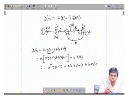
Okay, so if you see a signal flow graph or data flow graph, it does not matter how you draw it here now. The signal source it is generating x of n then you are it multiplying it by a factor. Then you can put a b here, b. So b into x n, then you add b into x n plus this is the plus and a into something. So there is a multiplier with a, a into whatever comes, maybe y n minus 1 comes that into a. When you add with this, this would be by this equation y n.
