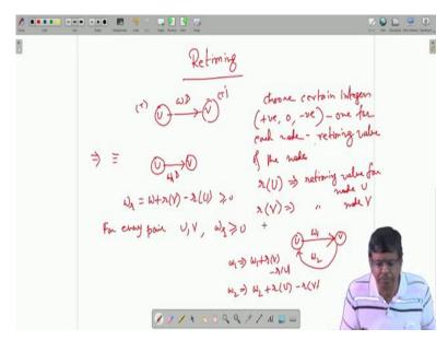
So the previous class we started with retiming and quickly what we did is these we said retiming is a method by which you can change the delays or the various edges in a giving data flow graph, maintaining equivalents. That is the new DFG you will be doing the same job at every node as the original DFG was doing. But this gives a formula to change and that is retiming and there I said that every sector of DFG if you pick up it will be of this type.
