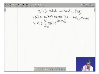
And this is done by a method called distributed arithmetic. In DSP you come across linear combinations like say, when we have a filter FIR filter. Output is W0 x n, W1 xn minus 1dot-dot-dot any W and just FIR filters. It is a linear combination, it has got so many multipliers, W0 into xn.
