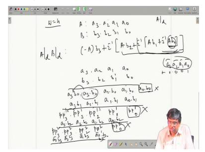
So the last class we are considering multiplication of two numbers using Horner's Rule and numbers were represented in two's complement format. We explain the Horner's rule, the chain rule and then we took a special case of 4 bit numbers. What is capital A, what is B, I applied Horner's rule and then led to a tabular of multiplication where you are truncating, I mean throwing LSB and then there is a sign extension and all these things and that is how you get the final result.
