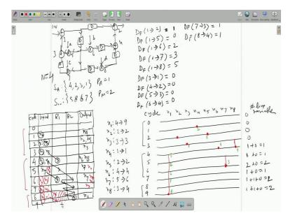
So, in the last class we are considering the delay optivation for this digital filter which we have studied earlier in the context of general folding there is the folding the multipliers and adders. So, all these figures were known to us we opt out this DF u comma v, u arrow v that is the folded delay expressions.
