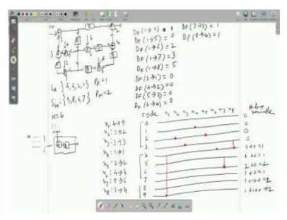
Adder 1, adder 2, adder 3, the same will stop 4, multiplier 5, multiplier 6, multiplier 7, multiplier 8, okay. The schedules were this, that is the folding sets SA was 4, 2, 3 1, SB sorry SM multiplier that was 5, 8, 6, 7 pipeline latches, PA was 1, PA was 2, okay, and period was 4 that as you read the input cycle system is working at 4 times faster than the input because folded by 4.
