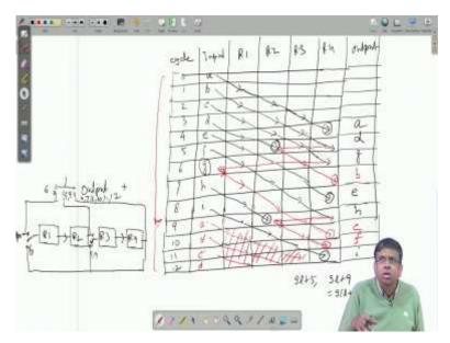
So I come back to this figure. So let us consider b, b got halted here, but you see in the very same cycle this fellow d is consumed, okay d is consumed, I do not need to propagate it further down the line. So R2 output was free or R3 input, R3 input is free, from R2 output I take it to the output port, I will not give it to the input of R3.
