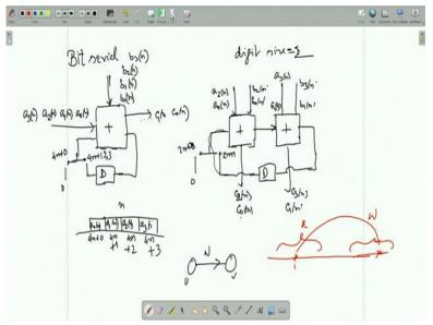
In the previous class we are considering bit serial, digit serial at word serial structures. As an example I took four bit full adder, which was working on fully word serial basis that is, four for one input a, full length for one input b, you are coming in parallel. All the bits, four bits of a, four bits b, and output four bits were going in parallel that is a fully word serial or b parallel structure.
