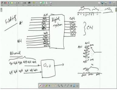
To continue suppose I have got a digital system, it takes two input A data and B data. A data maybe like this, 6 lines. So this is A, so LSB a0, you can write as a function of n in an n th clock, n th data clock. I have got input data An, whose 16, 6 bit depended are like this a0 th, which is a binary bit, either 1 or 0.
