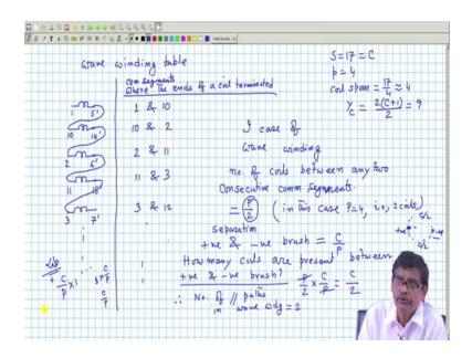
Let me come to this winding table wave winding table. For what I am doing the table? S equal to 17 which is equal to C, p is equal to 4, coil span is 17 by 4; I have to get an integer otherwise I cannot do anything approx chosen 4 and winding commutator pitch is 2 C I have taken plus for the earlier plus 1 by 2 I have taken which has come out to be 9.
