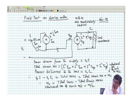
I will just mention another test that is called field test and it is carried out for D.C series motor fields test, fields test ok. Here, test field test on series motor. Here once again you require two similarly rated machines. For example, you have a series motor here, this armature, this is the field of the first machine ok, this will be connected like this.
