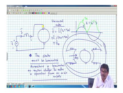
This is the field, this is the this one, it is a series motor; this is series motor. In this case, if you apply an AC supply, I do not care, because this current; armature current and field current are same and they cannot, but change together. That is in this case; both armature current and field current are same and their indistinguishable. Therefore, if I is like this; this is I suppose I say, small i better indicate if it is to be operate i. This i is nothing, but i a nothing but, i field.
