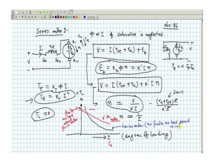
And, we have seen that in case of DC series motor the armature is as usual, but there is the field winding which are having fewer number of turns that is why I am just drawing like this only few turns and field terminals are marked as S e 1 and S e 2 and these two are as usual armature terminals and what happens is this, the field winding is connected in series with the armature.
