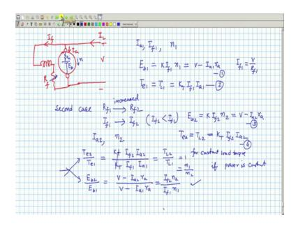
This is the DC motor armature and this is your field circuit, ok. This is the field circuit optimum motto, this is the armature current it is drawing, this is no, this is line current always show correctly and this is the armature current I a and this is field current at some value of field current and this is the field resistance generally. Now, suppose this is the voltage, initially steady state operating point only I will tell.
