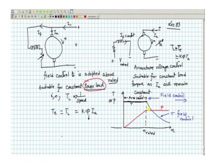
And, there are two very important methods. In which one method where armature voltage is varied keeping field current constant, I will not touch field current, it will constant remain constant and I will vary armature voltage from a variable dc supply voltage. And, then I found that if the load torque is constant. Then armature current will remain constant no matter what armature voltage you have applied. And, therefore, it will be suitable for constant load torque drive.
