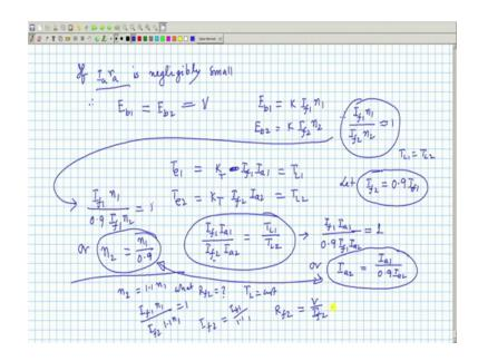
If it is neglected so approximately you can say that, if r a is; I r a is negligibly small, which will be small only negligibly small, then a your E b 1 and is equal to E b 2 is equal to V, there ends the matter is not. And, E b 1 was equal to K I f 1 into n 1 E b 2 was equal to K I f 2 into it was there. And, therefore, I get I f 1 n 1 is equal to I f 2 n 2 and that will be closely 1 that which has to be.
