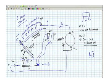
Last time I told you about a very popular; it is to be a very popular starter for shunt motor. The ideas were given starter is a device which protects the machine from very high current drawn at the time of starting, because of the absence of any back EMF. So, you insert a resistance in series with the armature, then gradually cut out and finally, it will be running with full voltage across it is armature and field supply.
