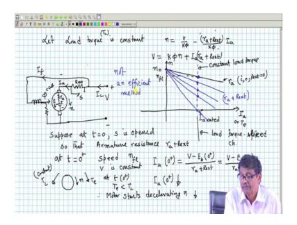
So, let load torque is constant, ok. Load torque T L and this is the circuit diagram, I will just take this circuit diagram here so, that I do not have to do. So, this is the same diagram let me put it here and armature and field. Now, I will not make R external 0, suppose machine this is the general equation of the armature voltage V is equal to K phi n plus I a r a. And, will r a plus R external. Now, let us try to understand why speed will change rather physically what is happening?
