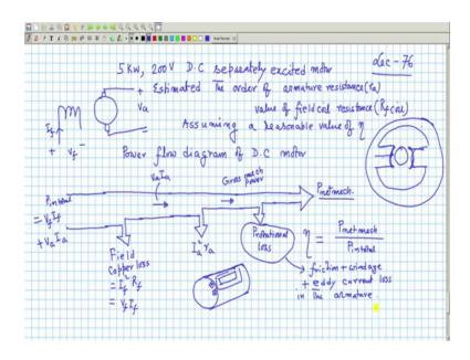
And suppose I took a DC machine name plate rating as 5 kilo watt, 200 Volt I have taken it will be 220 Volt may be for easy calculations. DC separately excited motor; DC separately excited motor. We were took this motor to explain the things.
