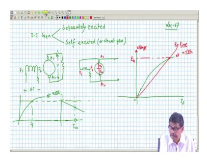
And DC generator primarily are of 2 types we have discussed, one is a separately excited generator and another is called self excited or shunt generator self excited or shunt generator. Why it is self excited? You do not require any DC supply applied that is to generate a DC voltage you will not ask for another DC supply needed that is the beautiful thing about self excited generators or shunt generators ok.
