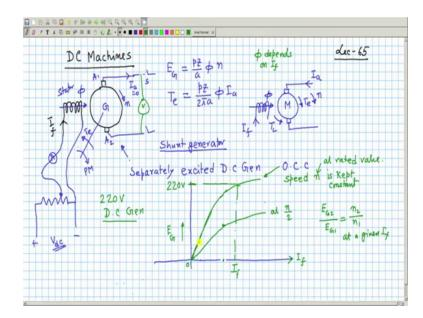
As you know these are the brush and these are the; this is the field coil, that is all and field coil to be excited from a separate DC source. When it is separately excited, DC machine I f and suppose, when field current flows like this, the flux produced per pole is in this direction, this is called phi and these two are armature terminals, which will be like this and these are the four terminals, which will be available to us.
