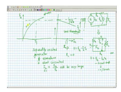
So, we have got these no load voltage, this was the OCC, this was E G across the armature and this is suppose the rated voltage and this is the field current, there is the normal field current and OCC whenever you draw you must specify at what RPM at n r p s. So, this is about this and what is the connection diagram. Keep it in your mind that this is the diagram which is relevant now.
