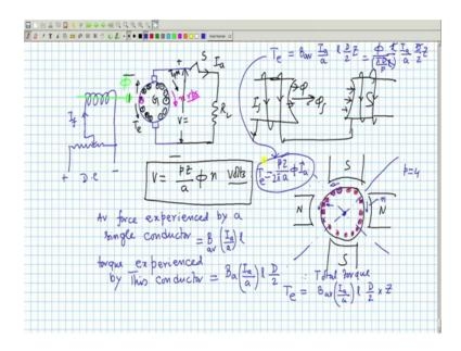
This is suppose the field winding we will now refer to this simplified diagram and this is your armature terminals, you pass some field current please try to follow me. Suppose this is the I f and because of this I f where you have connected perhaps say potential divider connection you do and you can vary the field current also plus minus you require a DC source like that and it is a separately excited DC machine field winding is excited.
