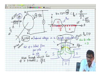
My goal was to find out what will be the voltage available across the armature terminals when no load is connected open circuit condition we have passed a DC current in the field winding it has produced a flux per pole phi then my question was what will be the voltage induced in that. I know brush between the brush there will be several circuits in parallel that is all the armature conductors will be divided into several parallel pass.
