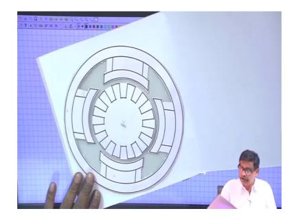
So, if you see that these are the poles stator poles where there will be coils around it to create north south; north south and this armature it is slot and teeth slot teeth where the conductors will be placed and this whole thing has got a length perpendicular to the plane of the paper and this fellow will rotate and the conductors which will be placed here will be the armature winding ok.
