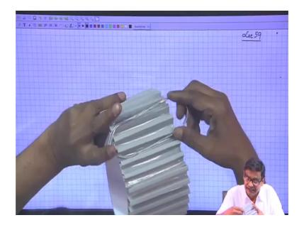
See this is the actually this will be the rotor are you getting? This way and it is because the rotor windings is the most crucial in DC machine stator windings are very simple there will be 4 coils, if it is 4 pole machine and these coils are to be connected in series and ultimately 2 terminals will come out they are called field terminals, which is to be excited by some DC current creating north south north south poles but the armature winding is rather interesting.
