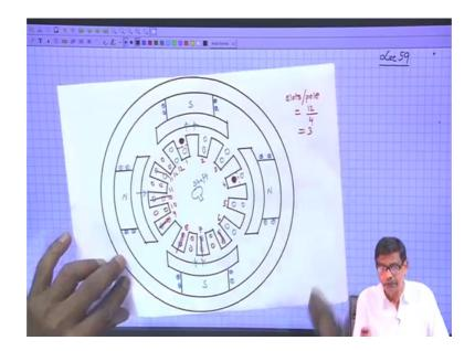
So,. So, this is the thing and if you look at this diagram on a paper the same diagram I am telling, what is to be done is that this stator poles will be created by conductors placed around it is not and suppose this carries cross current and this carried dot current then this becomes a north pole.
