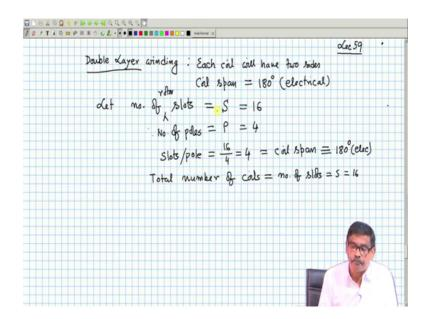
Now, what I will tell you is this that, now we will be talking about double layer windings double layer winding ok. That is each slots conductors will be placed on slots each coil will have two sides and we will assume coil span is equal to 180 degree electrical and this I have to do in order to maximize the voltage that is what I explained in the last class.
