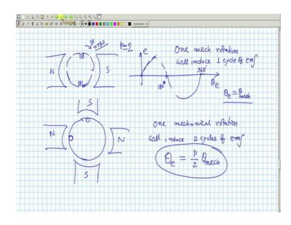
But nonetheless I explained to you that in a DC machine there will be a stator structure, which will have projected poles like this and it could be a 2 pole or multipolar stators this north south poles will be created by coils, which will be put around it these are called field coils and on the rotor side there will be an armature.
