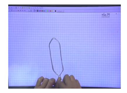
So, this is a coil which is diamond shaped like this, it is a coil like this and this coil has got 2 coils sides. If at any time these coil side will be under north pole the other will be under south pole. So, how this coil will be placed? It will be placed in its designated slot
