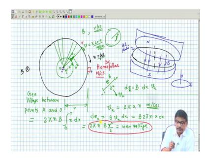
And, recall that in my last lecture I told you about a simple type of DC generator, where an aluminum disk is rotated at some given rps of certain radius r. And, there will be magnetic field from top to bottom penetrating the disk, all over the surface of the disk. Then, what happens is if you consider a radial line, there will be induced voltage between the center and the perimeter of this disk. And, the value of that voltage is given by this expression ok, this expression.
