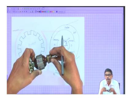
But, armature will be a bit complicated we will come to that and before that I will show you a an actual DC machine armature a small DC machine armature.
