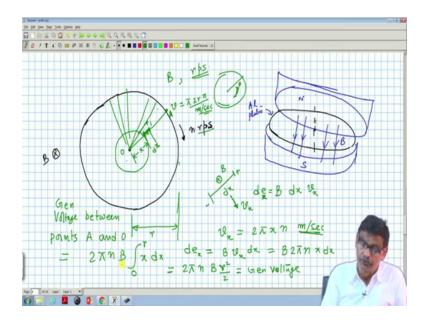
Aluminum disc and a circular aluminum disc and it has got a spindle about which it can be rotated vertical axis along this line that is there. Now, on the top you keep a north pole suppose this is a north pole above it ok.
