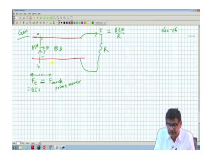
Suppose you have a generator on this railway track as we have drawn earlier and very quickly I can write down the results this is my a b conductor generator mode generator and it is running initially with velocity. And suppose I say like this it is running with velocity v at constant speed and then I say that the generator is supplying a resistance like this and your b is in this direction. So, polarity of the voltage induced will be Blv is it not.
