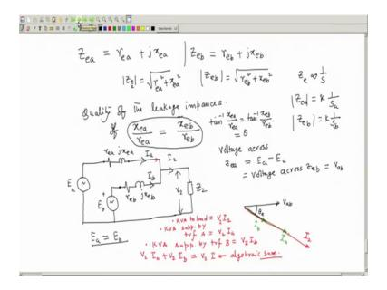
Welcome to 50th lecture on Electrical Machines – I, and we have been discussing about Parallel Operations of Transformer. So, we have seen that in our last class the impedances of leakage impedances of the transformer should be inversely proportional to the KVAs and in ohms and also of the it is always better if the qualities are also same. Then, whatever KVA is supplied by this, whatever KVA is supplied by transformer be just algebraic sum of this two will come.
