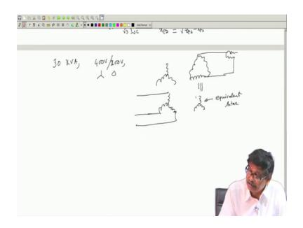
Now, suppose I say that the transformer is star delta, ok. Same rating what I told 30 kVA. Suppose, I say that 30 kVA, 400 volt, 200 volt, and the connection is star delta then what do I do? How to draw the equivalent circuit like that? Ok. You have to carry out the open circuit and short circuit test. Because the readings we are taking are only the line readings, is not. We are while carrying out the test I am measuring the line quantities.
