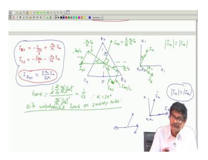
So, it was like this, a 1 b 1 and this is a 2 b 2 and primary phasor diagram was like that A S, B S and C S and this was the point O it was like this. Now, these currents where you recall I a and this current was I b their lengths are same, because balance load I have assumed and this is the power factor angle theta 2.
