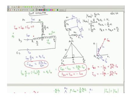
And for this you required 2 transformers ah, one transformer is B 1 B 2 and its corresponding secondary terminals is also b 1 b 2 and an another transformer which is a separate transformer of terminal markings capital A 1 A 2 and small a 1 a 2. What is the thing we discussed that the number of turns of the secondaries are same.
