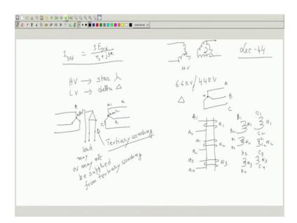
This 3rd harmonic current will circulate like this. So, 3 times E 3rd divided by the leakage impedance of this side, but if the at the fundamental frequency leakage impedance is x 1 it should be j 3 x 1. So, impedance also increases and there will be
