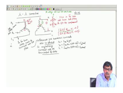
In case of say star star connections without neutral connected anywhere no scope for any third harmonic current to exist in the lines of this transformers and therefore, the flux must be having a 50 Hertz as well as 150 Hertz component; other higher order harmonic components are also there, but we are neglecting that because their amplitudes will become smaller.
