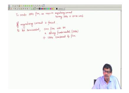
Remember that these are the two things that is, if magnetizing current happens to be sinusoidal 50 Hertz then core flux will have both 50 Hertz and 150 Hertz component ok. On the other hand if the flux in the core is 50 Hertz only then magnetizing current must have 50 Hertz component as well as 150 Hertz component, then depending on situations the current may not have a 150 Hertz component.
