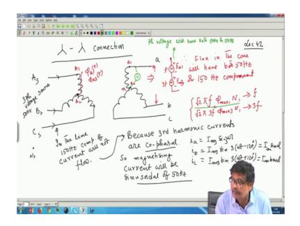
Now, today I will discuss for example, take the star-star connection of a three-phase transformer ok. Now, continuing with that so, consider start star connection of three-phase transformer and this connection can be obtained by using three single phase transformers or a single three-phase unit transformer first let us see that, but the connections are same in both the cases. So, suppose I will simply draw like this now because we will presume that whoever is connecting is connecting correctly.
