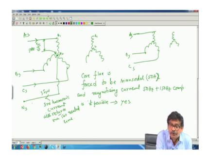
Suppose, I say that this is the primary star this is the secondary and for a change what I will do this is A s I wrote this is B s B s 1 I wrote like that. So, anyway so, this is B s I wrote is not B s and this is C s I have drawn and the supply neutral listen to this point also I have connected to this primary neutral.
