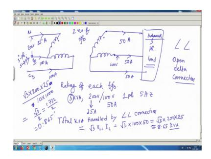
In other words in simplified diagram, what I am telling; suppose you what you have essentially done is, which transformers I have removed. If I draw it in a simplified diagram, I will do it like this; this is one transformer, this is another transformer, this is it secondary, this is it secondary and the third transformer is not there. And what I have done, I have connected 3 phase supply there A s B s C s, 3 phase supply.
