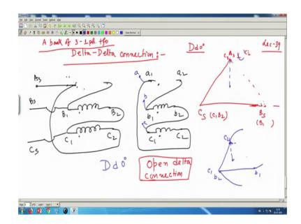
And we were discussing use of 3 single phase transformers to step up or step down voltage it depends upon the connections, what will become the line to line voltage, transformation. And also we have fairly understood what is the phase shift of the secondary voltage with respect to primary voltage and what are the possible connections familiar conditions like star delta, delta star, delta-delta and so on.
