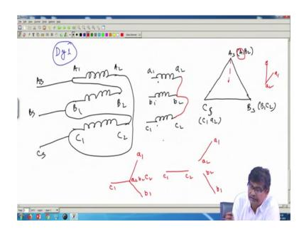
Suppose I now say that connect Dy 1 the connection I know now. The point I want to make it is interesting you see this is the 3 transformers you have A 1 A 2, this is B 1 B 2 and this is C 1 C 2 good and this is secondary small a 1 a 2 one terminals are dot terminals which I am not writing all the time b 1 b 2, c 1 c 2 fine. Then what I am telling you connect this as delta like this for example, same thing I am doing I mean do not worry this is As this is supply Bs and this is supply Cs.
