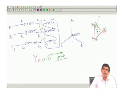
And let us see another connection for example, star delta I will make, but delta this time I will go other way around for example, this is A 1 A 2 this is B 1 B 2 and this is C 1 C2 these are dots not these and these dot we are talking about each secondary dot that is each secondary these are three separate transformers no question of mutual drop. So, this is dot b 1 b 2 and this is c 1 c 2 this is also dot.
