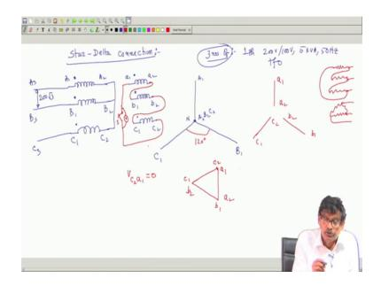
Welcome to lecture number 36 and we have been discussing about the 3 Phase Transformer Connections. Recall that last time, I was discussing about star delta connection. And referred to this diagram, where the primaries are connected in star SV side applied voltage is 200 root 3, then I told you when this 3 coils no connections with this red markings have been made. Then these phasors will maintain their 120 degree phase difference, but they will be in isolated conditions they are separate.
