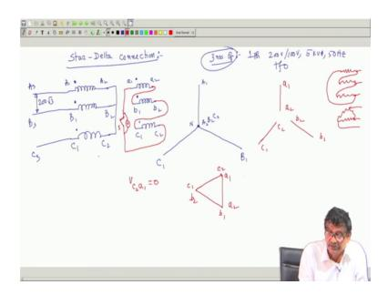
So, I take suppose I want to do star delta connection of the same 3 phase transformer. So, once again follow me follow these steps, draw the coils A 1, A 2. Each secondary small a
