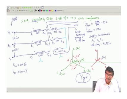
And I showed you a simple star star connection ok. The terminals markings are essential, along with polarity marking. So, I have assumed because three transformers are there, I will name them A transformer B transformer C transformer. Capital A 1, A 2 small a 1, a 2 are the are respectively high voltage and LV side terminals and I have presumed that this 1 1 are the dots for all the phases so that is there, so they here also it was taught anyway.
