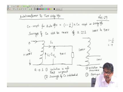
Welcome to lecture number 29 on Electrical Machines I and we have been discussing Auto Transformer. In fact, we have been comparing auto transformer versus two winding transformer, two winding transformer.
