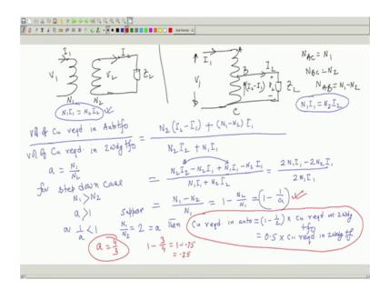
So, it looks like copper required in autotransformer rather volume of copper required, volume of volume of copper required, volume divided by volume of copper required in two winding transformer I am trying to finding. Now, what is the number of turns, length of these wire will be proportional to N BC, is it not and N BC is N 2 into the cross sectional area proportional to the current.
