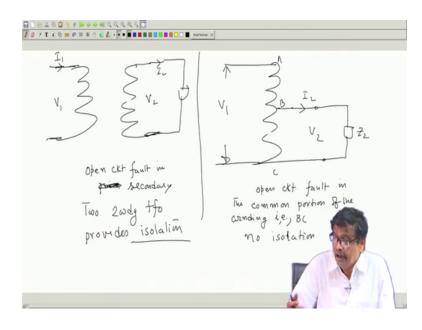
For example, I will tell you that suppose you have an two-winding transformer, V 1 V 2 you are getting. And a similar rated auto transformer where V 1 and V 2 you are getting that is fine. A two winding transformer, suppose let us consider a situation, it is supplying load ok, it is supplying load, connected rated current it is supplying that is what I would like to operate the transformer because I have purchased a transformer of given kva let it handled given kva why operate it under no load.
