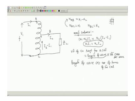
So, I draw the transformer once again. So, this is the auto transformer which step downs the voltage V 1 AC voltage. This point I call A, this point is C and here is the tapping B, and here is the load connected get to secondary load. And this was the current distribution I 2, this was I 1 and then this current was I 2 minus I 1. This number of turns N AB N AC is equal to N 1 this total number of turns N BC is equal to N 2 turns.
