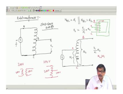
So, autotransformer it is like this, this is the coil I will draw this way. And here is your tappings taken, I will say this terminal as A this terminal is C indicating common between primary and secondary. And I will say that N AC is equal to N 1 and here I will apply voltage of frequency f.
