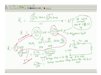
And we found that the regulation is given by this expression ultimately we derived. It could of course, be expressed in terms of either primary and secondary. So, with respect to primary side regulation turns out to be I 2 dashed r e 1 by rated voltage cosine theta plus I 2 dashed x e 1 by V 1 these are magnitudes this is an algebraic equation and cos theta is the power factor of the load, then I told that this quantity I 2 dashed by r e 1 by V 1 is called the per unit resistance.
